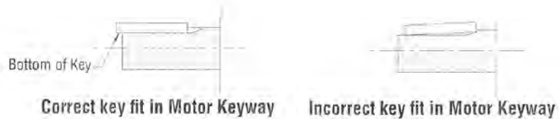
Figure 5 - Clamp Collar Motor Key Fit
